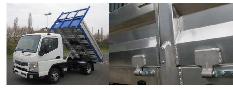
Tipmaster uses aluminium sheet for tipper floors and headboards, and aluminium planks for the sides and tailboard, making bodies 23% lighter
